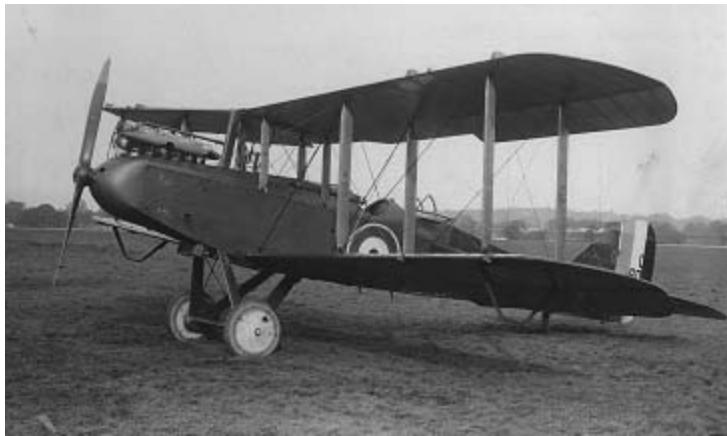
DH9 Aeroplane. The pilot's Vickers machine gun was located in a recess to port. The large object clearly visible on the engine is the exhaust manifold. ( Royal Aeronautical Society )
